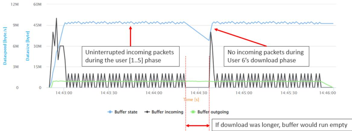
**Figure 4: Example FAIL case during the download burst**
