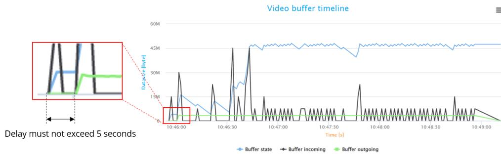
Figure 5: FAIL case for video start delay
